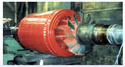
Metallise & grind on shaft bearing & seal areas.
